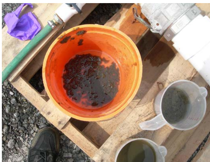
The sample port was used to collect conditioned residuals to verify polymer dose prior to transfer to the Geotube® container.
