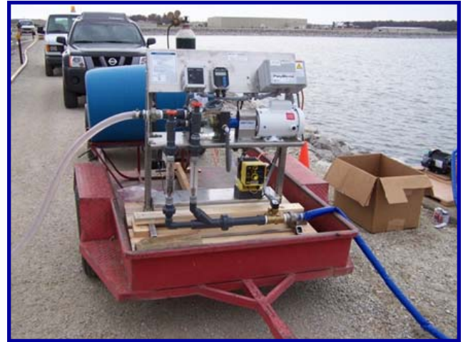
WSLP-2400 polymer make down unit for blending and calibrating polymer feeding rates.
