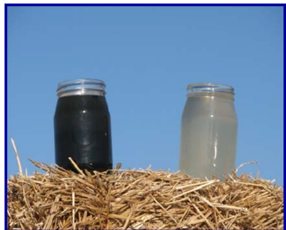
Dredged influent water on left. Effluent from Geotube® container on right.
