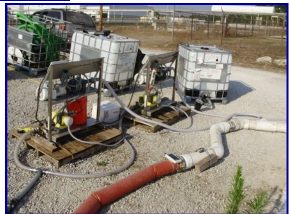
These two WSLP-2400 polymer make-down units deliver up to 20-gph of Solve 9330 to the 6" mixing manifold.
