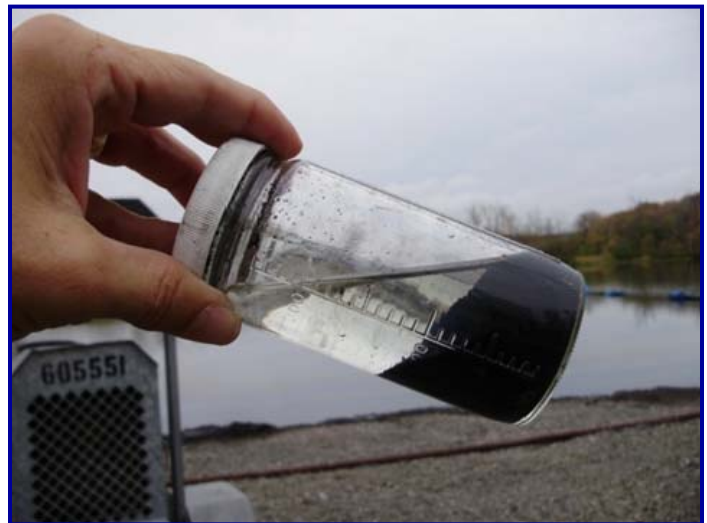
Lagoon residual conditioned with Solve 9248 at the project site.
