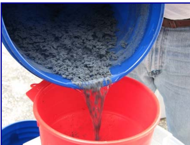
The chemically treated residuals showing great flocculation and water separation.
