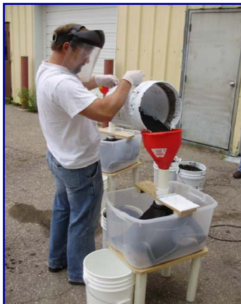
The water based adhesive residuals are chemically treated and poured into the GDT to collect filtrate for lab analysis and measure the dry-down rate of the cake inside the tube.
