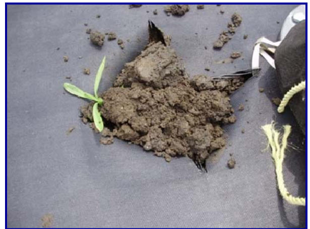
After being filled in October of 2008, a sample from the Geotube® container was taken, the dry wt solids were 15% which passed the paint filter test.
