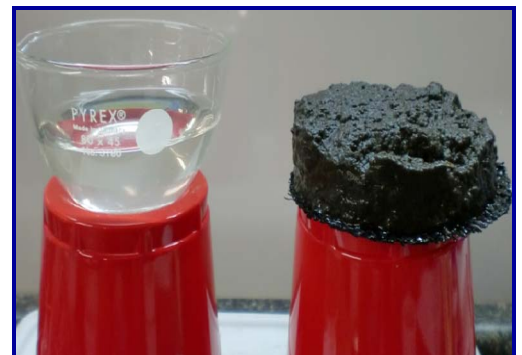
The 150-mL sample of biosolids was treated with Solve 216B then poured onto a Geotube® filter. The filtrate water is on the left and the resulting cake was collected at the end of 1 hour. The cake tested 6% dry wt. solids.
