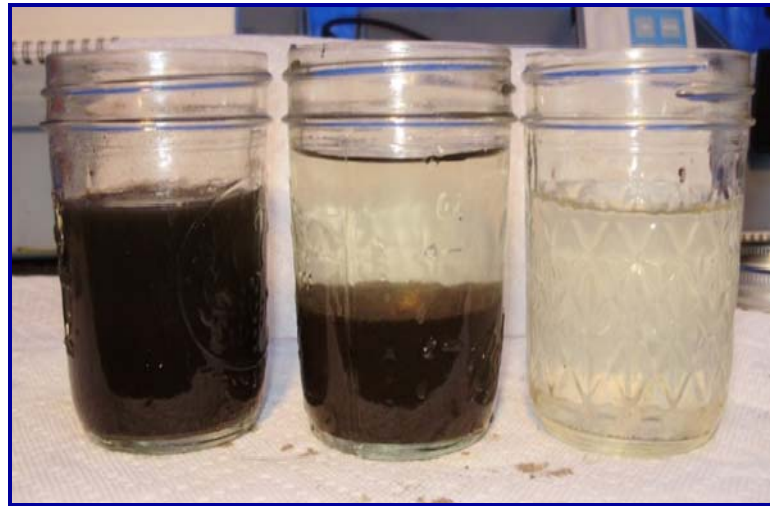
The raw dredge water is on the left, the chemically treated water is in the center, and the settled discharge water is on the right.
