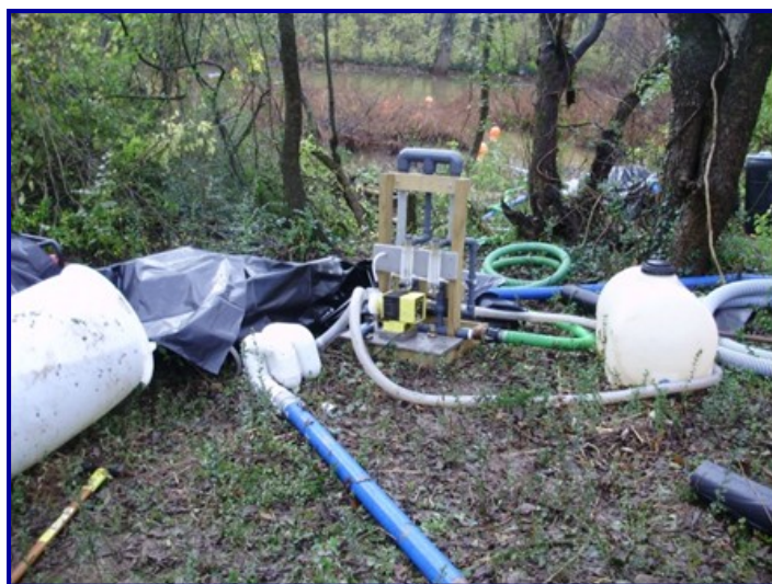
The flocculent Solve 164 is injected into the mixing manifold with WSLP 1000V2 polymer make-down unit .
