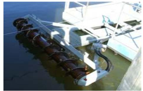
An Ellicott auger dredge was used to dredge the sediments in the waterway and in the boat slips.
