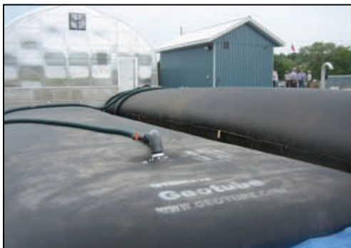
The Eganville facility features two outdoor dewatering cells (left) and a cold weather greenhouse enclosure (right) for year-round use of Geotube® dewatering technology. This accommodates Winter emergency pump outs.
