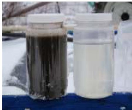
Filtrate from the Geotube® dewatering technology in comparison to the raw sludge which was pumped from the forebay.
