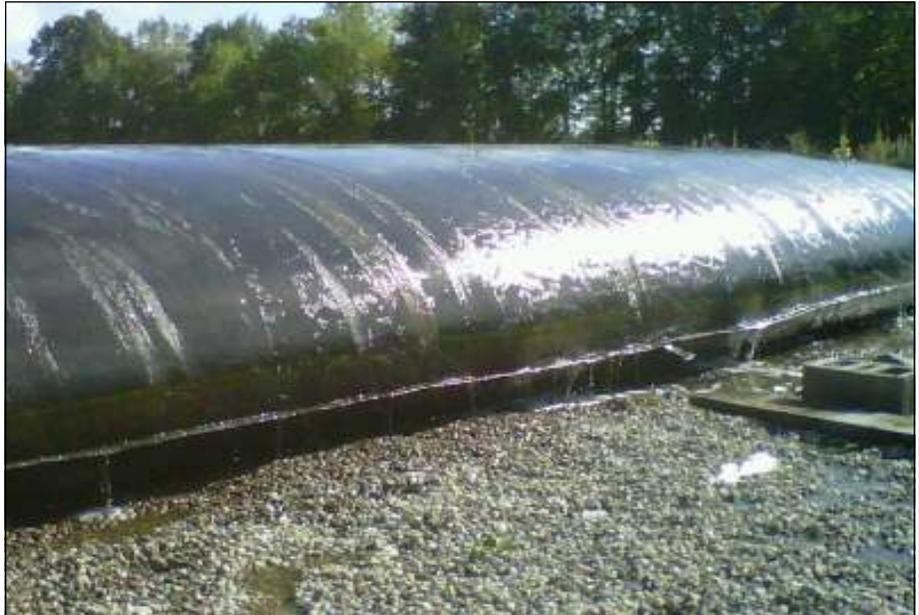
*As un-stabilized septage is pumped into the Geotube® unit clear filtrate immediately begins to flow from the bag at the Howard Campbell and Sons Geotube® Facility in Lyn, Ontario*
