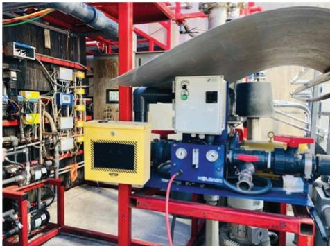
*Moleaer's 200GPM nanobubble generator is a far superior treatment system for MBRs when compared to conventional aeration.*
