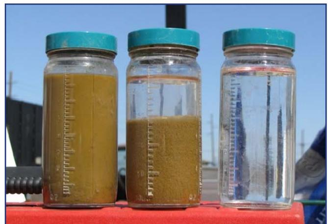
The raw dredged sample (left) was conditioned with 66-ppm of Solve 9330 (center). The filtrate collected from the Geotube® container is on the right.
