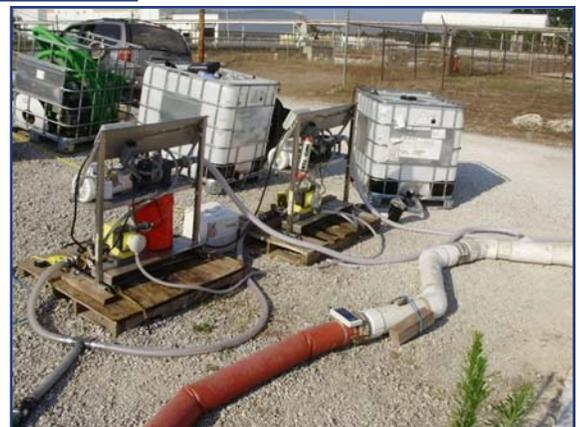
These two polymer make-down units deliver up to 20-gph of Solve 9330 to the 6" mixing manifold.
