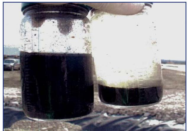
*In situ* sediment sample compared to chemical conditioned sediment.
