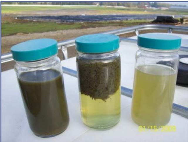
Photo shows raw sample on the left, chemically treated sample in the center, and filtrate on the right .
