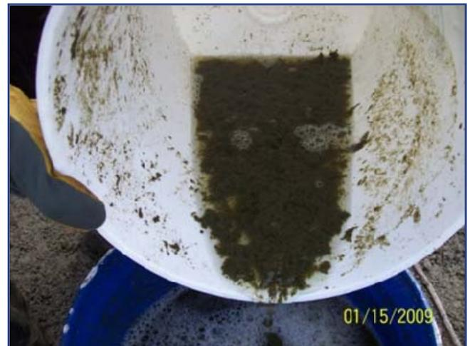
A chemically treated sample indicates good release, clarity, and flocculation of the dairy manure residual.
