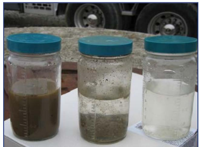
The sediment sample (left) was conditioned with Solve 9233 (center). The Geotube® filtrate is shown on the right.
