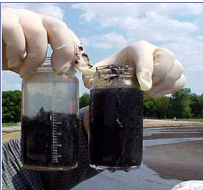
The South Lagoon residual chemically conditioned with Solve 9233 compared to unconditioned residual.
