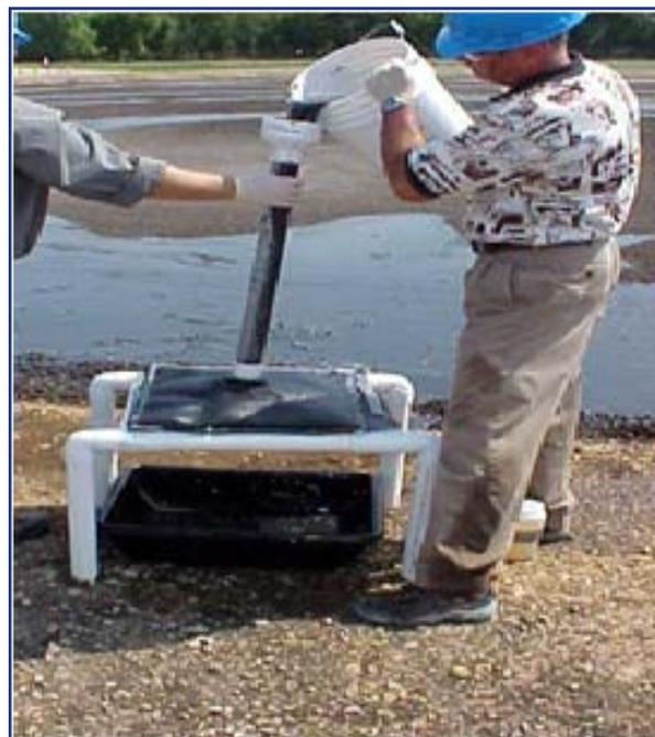
The oil-contaminated lagoon residual conditioned with Solve 9233 were poured through a GDT container. Filtrate and core samples were collected for drying timeline.
