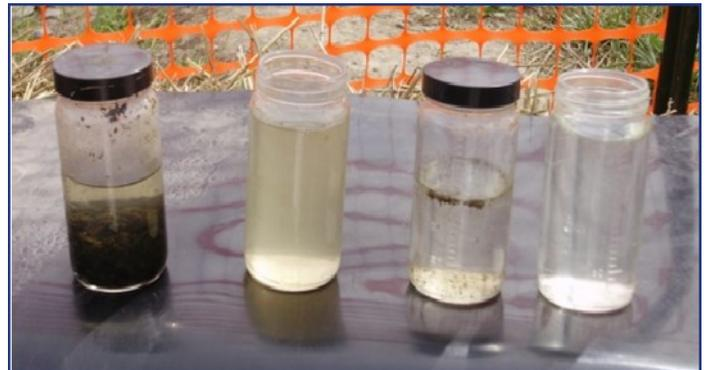
From left to right, the above jars show; the conditioned dredge residual, the effluent water from the dredge Geotube® container, the effluent after further treatment, and the filtrate from the polishing Geotube® container.
