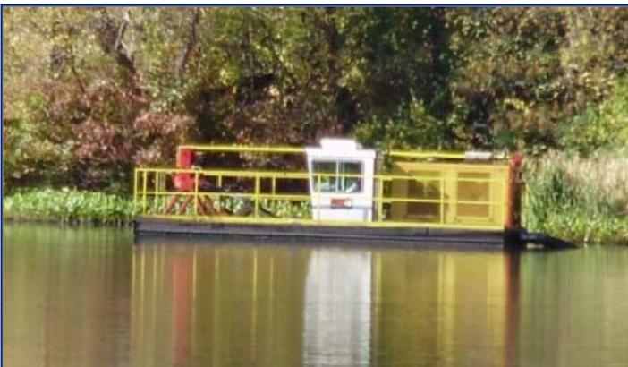
Dredge pumped at approximately 2,000-gpm with the assistance of an in-line booster pump.
