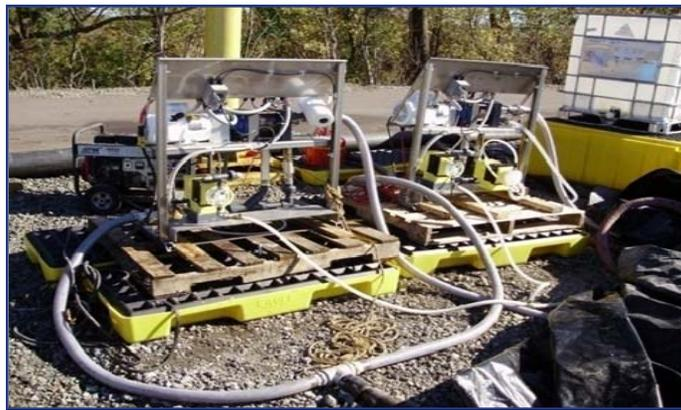
Note the lagoon is in the background. Piping and polymer make-down units and a polymer tote.
