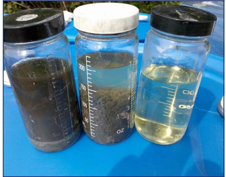
The chemical conditioning was verified periodically with jar tests. From left to right; the raw residual, the conditioned residual, and the filtrate collected from the containment area.
