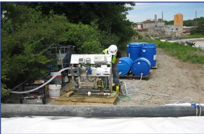
The chemical feed system is shown here. Two LMI metering pumps fed the Amerfloc 490 into the dredge line prior to the Drewfloc 2433, which was made-down and injected with a polymer make-down Unit.
