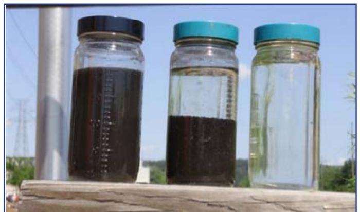
These samples from left to right represent the raw sediment being dredged, chemically treated with polymer, and filtrate water coming out of the Geotube® container.
