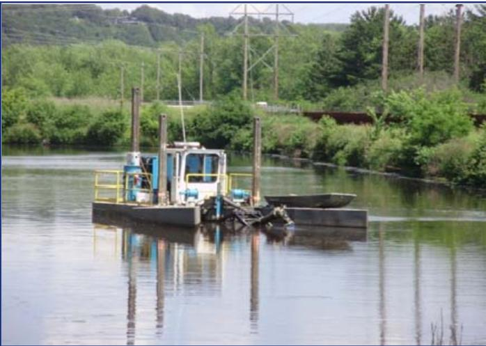
This hydraulic dredge pumped 1700-GPM of the sediment pond residual to the Geotube® containers.
