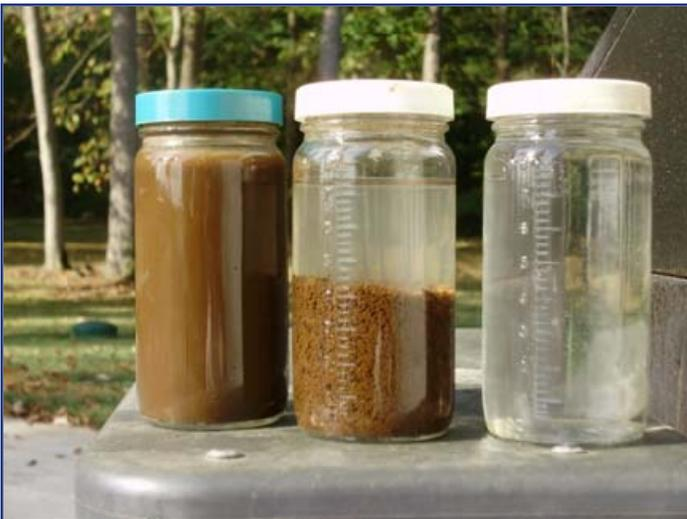
These jars represent the raw backwash water on the left, the chemically treated water in the center, and the filtrate water coming out of the Geotube® container on the right.
