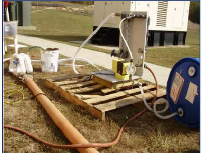
A polymer make-down unit is plumbed to the mixing manifold in the 3” supply line exiting the basin on its way to the Geotube® container.
