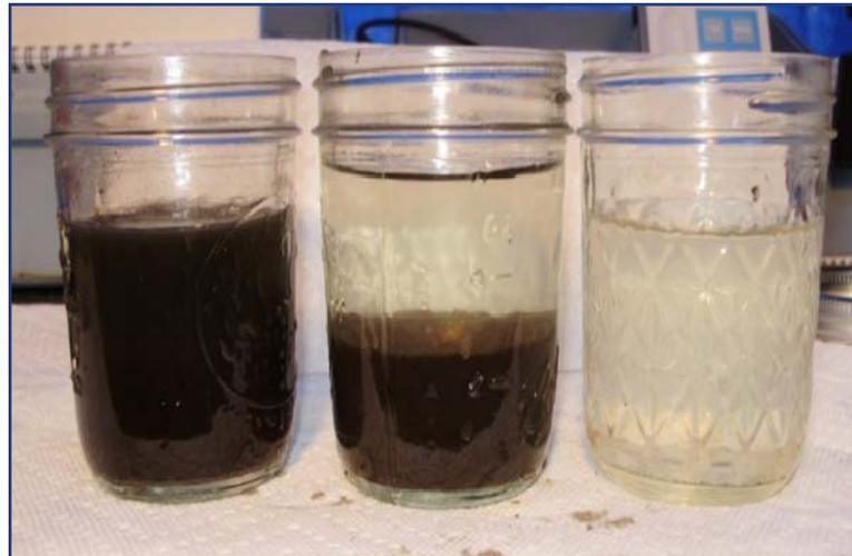
The raw dredge water is on the left, the chemically treated water is in the center, and the settled discharge water is on the right.
