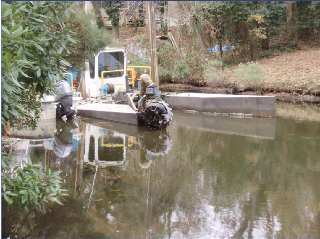
This hydraulic dredge dug through the canals and out into the sound sending the mud and sand to the lagoons at 2200 to 3000 GPM in a 10” pipeline.
