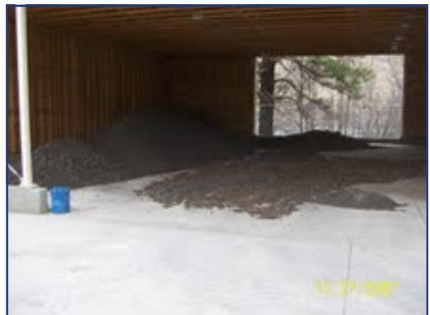
The sludge is drying after the Geotube® units are opened.
