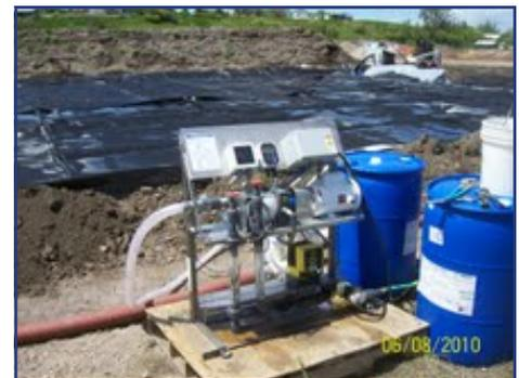
A polymer make-down unit for chemical addition and Solve 137.
