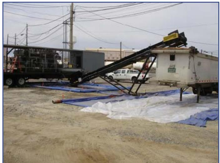
The hydraulic dredge dug the residuals from the settling pond and transferred them to mixing tank near the belt press. Then the belt press dewateres the residuals and the conveyor transfers them to the truck for hauling to a landfill.
