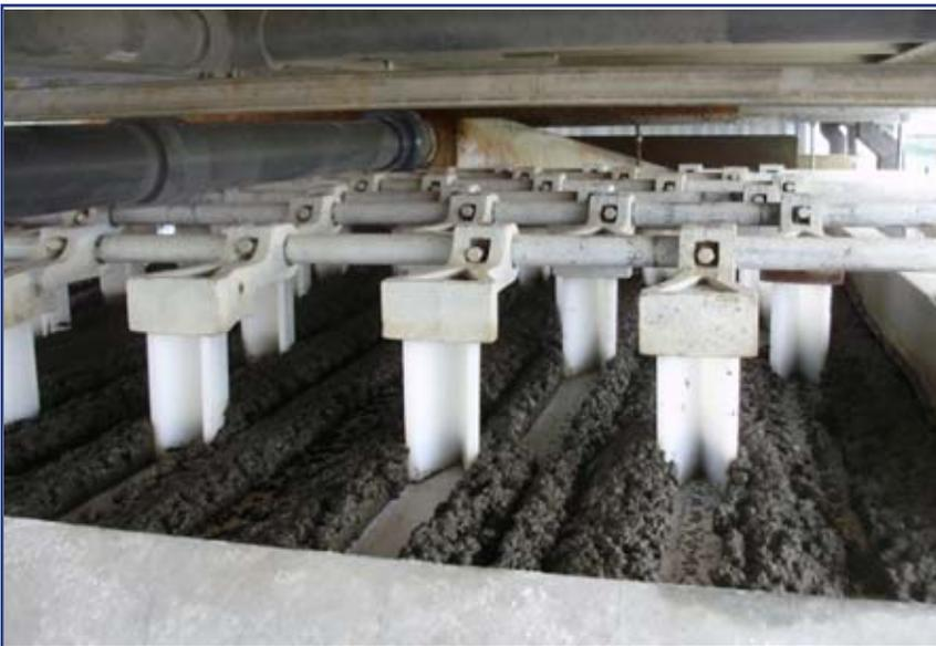
The Solve 137 polymer is working well as the dewatered pond residual is forming in nice straight rows on the belt press.
