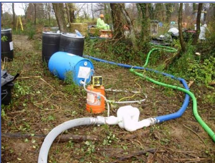
The coagulant Solve 426 is injected into the 3" mixing manifold .
