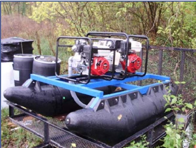
This Pirana Mini-Dredge has one engine to pump surface water to the dredge head for agitation and the other engine pumps the residual from the pond to the Geotube® container.
