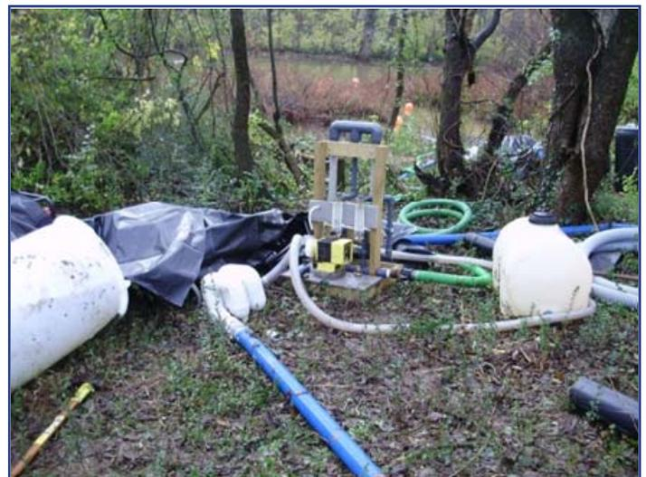
The flocculent Solve 164 is injected into the mixing manifold with the polymer make-down unit.
