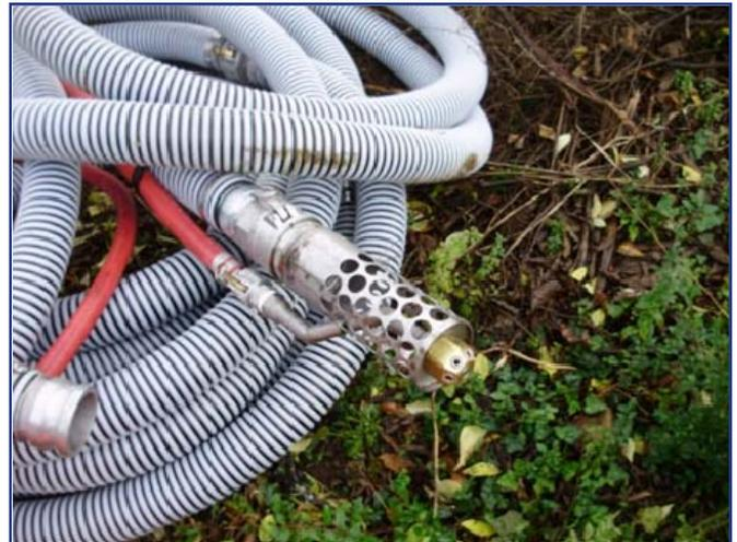
The red hose on the pump head delivers the agitation water to the spray nozzles and the strainer with the holes is the suction part of the dredge head.
