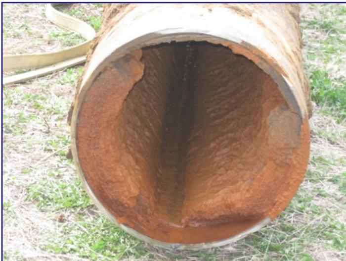
This cross section of the 12" pipeline showing the residual buildup that restricted flow to the water plant.
