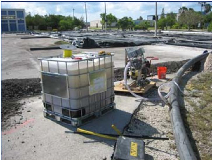
The polymer make-down unit is shown.
