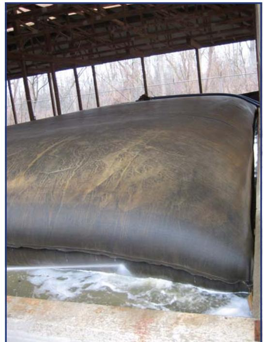
The Geotube® container during filling and dewatering operations.
