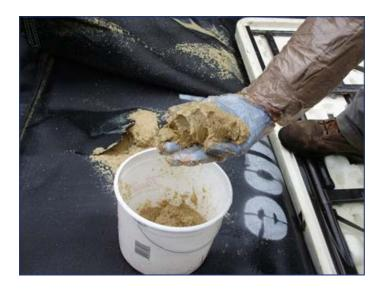
The residual was successfully captured as shown in photo taken 18 hours after the last fill which tested 11% dry wt. solids.
