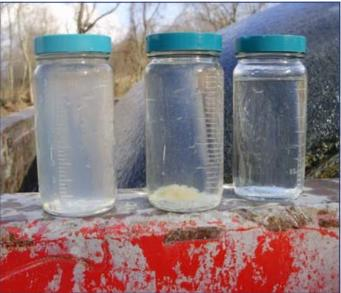
The water in this caustic mixing basin is raised from to 4.6 to 6.5pH which causes the cloudiness from the metals precipitating. A 3" electric pump transferred the water from this basin to the Geotube® container.
