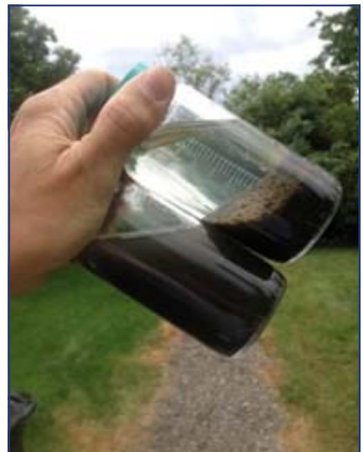
The bottom jar is without polymer treatment and the top jar demonstrates the clarity the Solve 137 polymer accomplishes in the settling pond.
