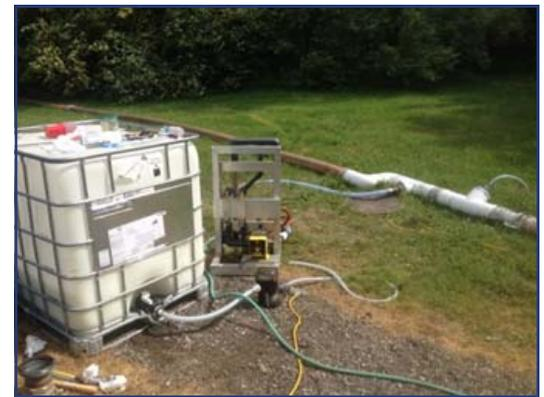
The polymer make-down unit is diluting the polymer with water and injecting it into the white mixing manifold on the right.
