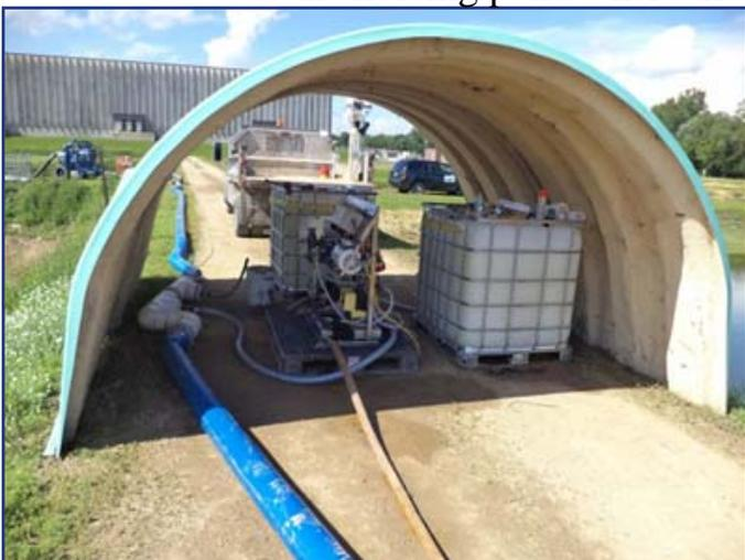
A polymer make-down unit dilutes the polymer and injects it into the biosolids pipeline. It was placed under the shelter with the polymer for protection from the weather.
