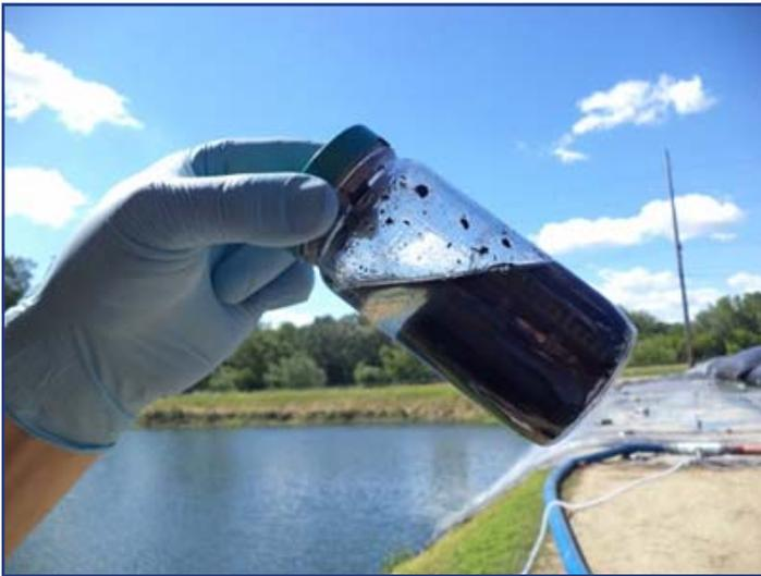
This sample jar contains the treated 2.8% biosolids being pumped.
