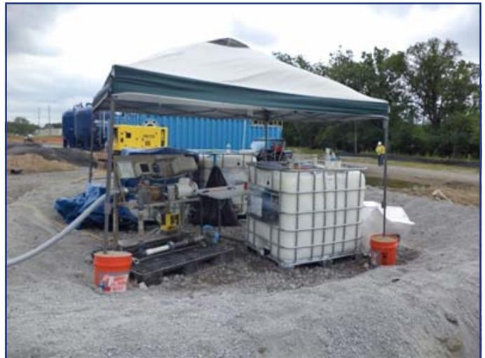
A polymer make-down unit dilutes the polymer and injects it into the dredge pipeline.
