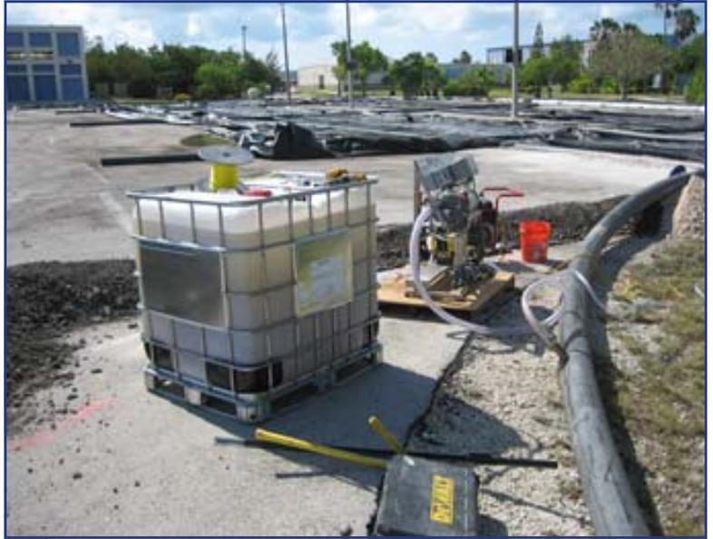
Above the polymer make down unit was placed on site and below the metering pump for Solve 426.
