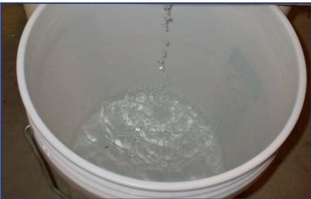
Above is the Geotube® Dewatering Test (GDT) apparatus. The conditioned sediment is poured into the container thru the riser pipe. The solids remain in the Geotube® container and the filtrated water is released and is collected in the bucket. This filtrated water was placed in one gallon containers and forwarded to an outside laboratory, for marine toxicity testing.
