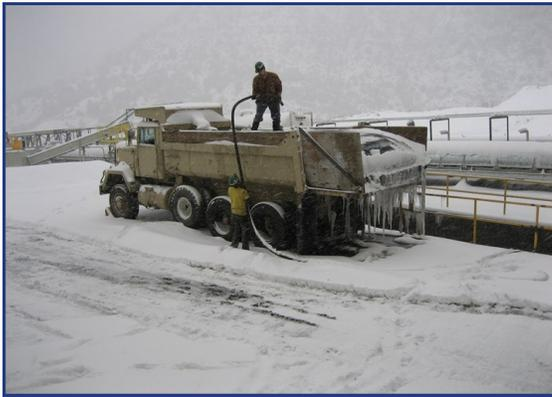
Significant snowfall was present at the mine area during the trial. The Geotube® container in the truck bed in the morning after pumping thickener feed all night. The filtrate is diverted into the sump area to the right and then pumped back into the plant.
