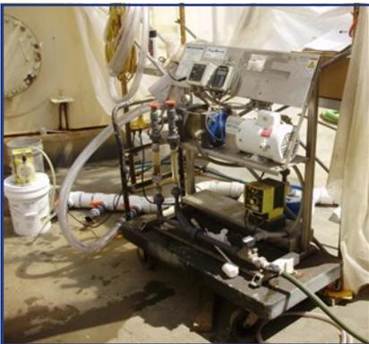
The LMI pump sitting on the pail in the left of the photo is injecting the Solve 7118 coagulant into the 2" residual pipeline. The polymer make-down unit in the center of the photo mixed the Solve 9330 with water and injected it into the pipeline as well.
