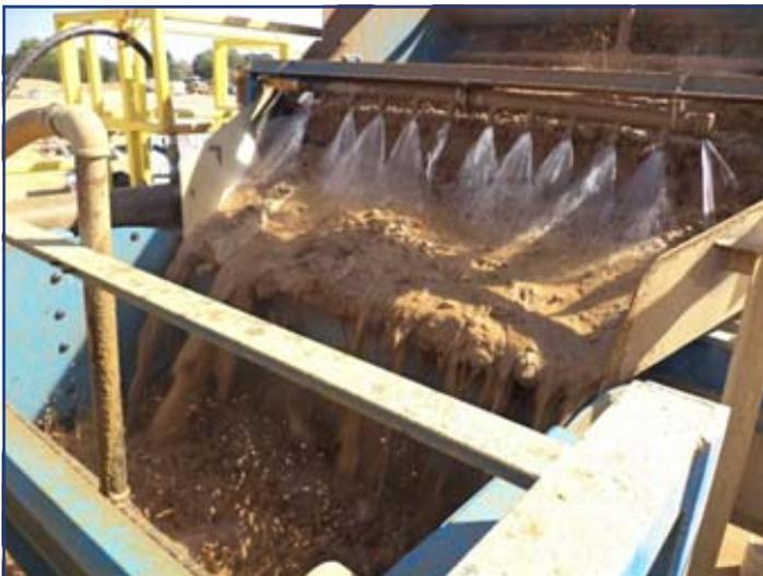
Water is sprayed on the sand as it goes across the screens to filter the sand in the plant.
