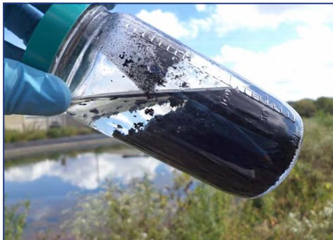
Sample jar of the residual treated with Solve 216B with great water release, clarity, and flocculation.
