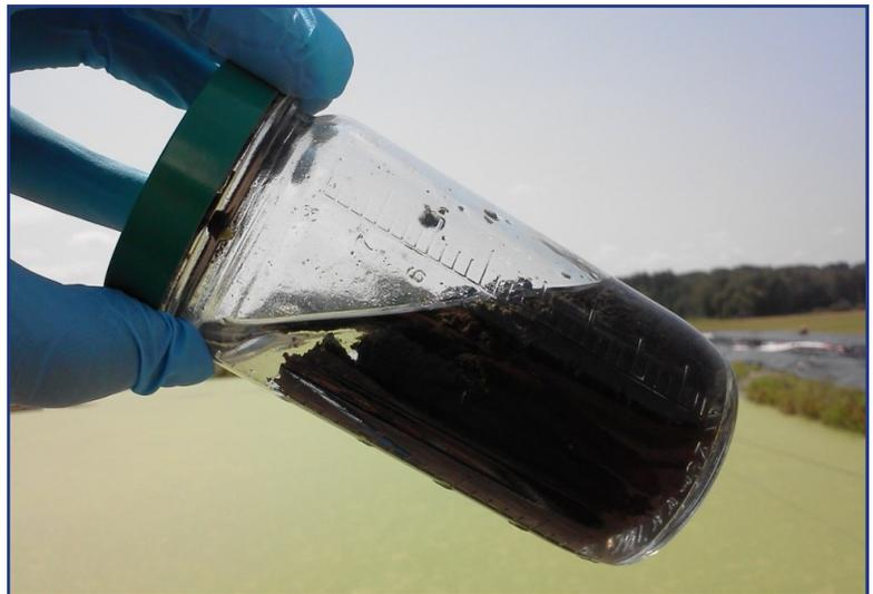
A sample jar of the residual treated with Solve 216B. It has excellent clarity, water release and flocculation.
