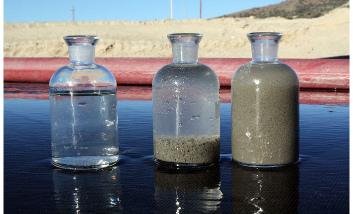
(Right to Left) Carbon fines, carbon fines conditioned with Solve 9330, filtrate.
