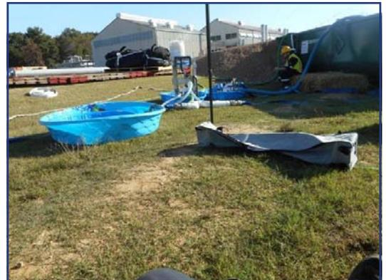
The polymer feed unit is injecting the Solve 163 into the pipeline in the center of this photo.
