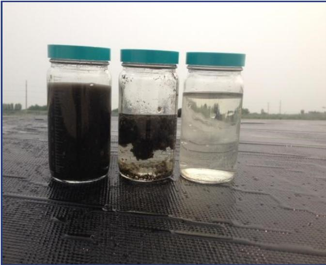
These jars represent the raw, treated, and filtrate samples of the potato residual. Notice the material floating in the center jar. This explains why the water releases from the bottom of the Geotube® container.
