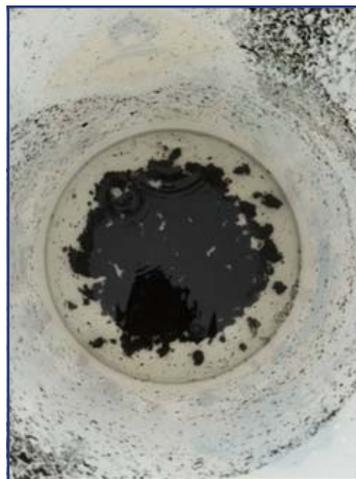
This sample demonstrates the proper flocculation with great water release.
