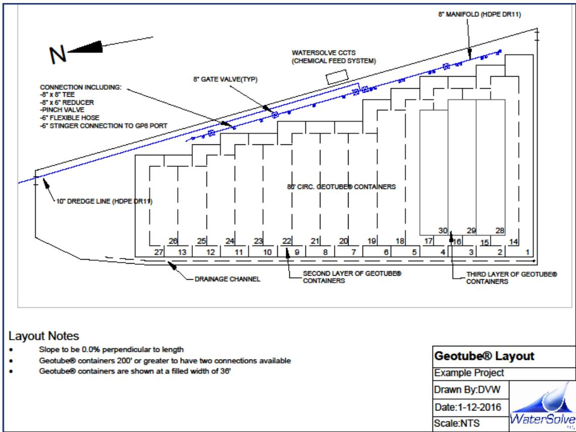
CAD drawings used to show Geotube® containers layout and piping configurations.
