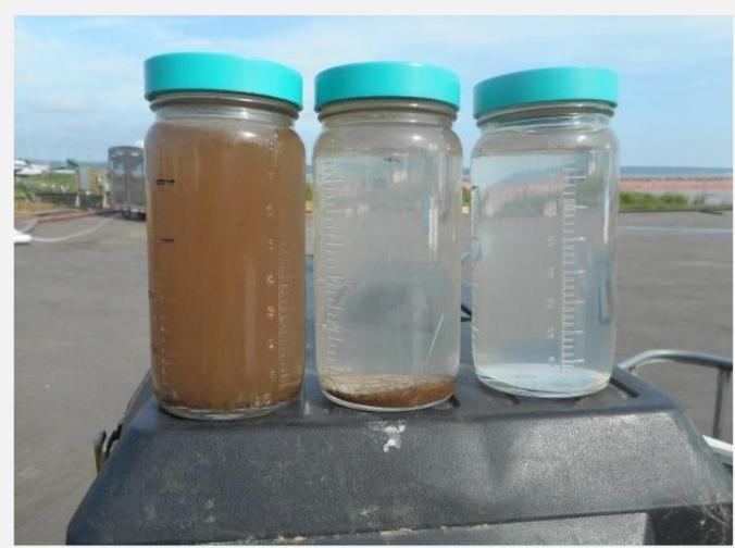
The jar on the left is the residual untreated. The jar in the center is treated with the Solve 426 and Solve 161. The clear jar on the right is the filtrate water coming out of the Geotube® containers.
