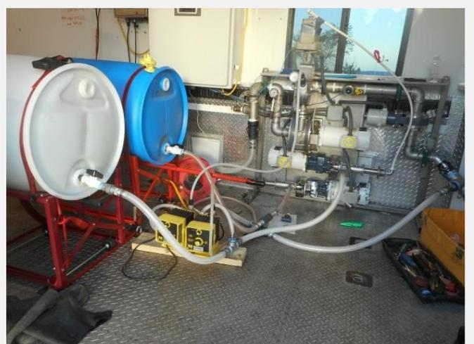
Two LMI pumps were plumbed into the polymer feed system in the WaterSolve trailer to deliver 3-ppm of polymer to the dredge pipeline.
