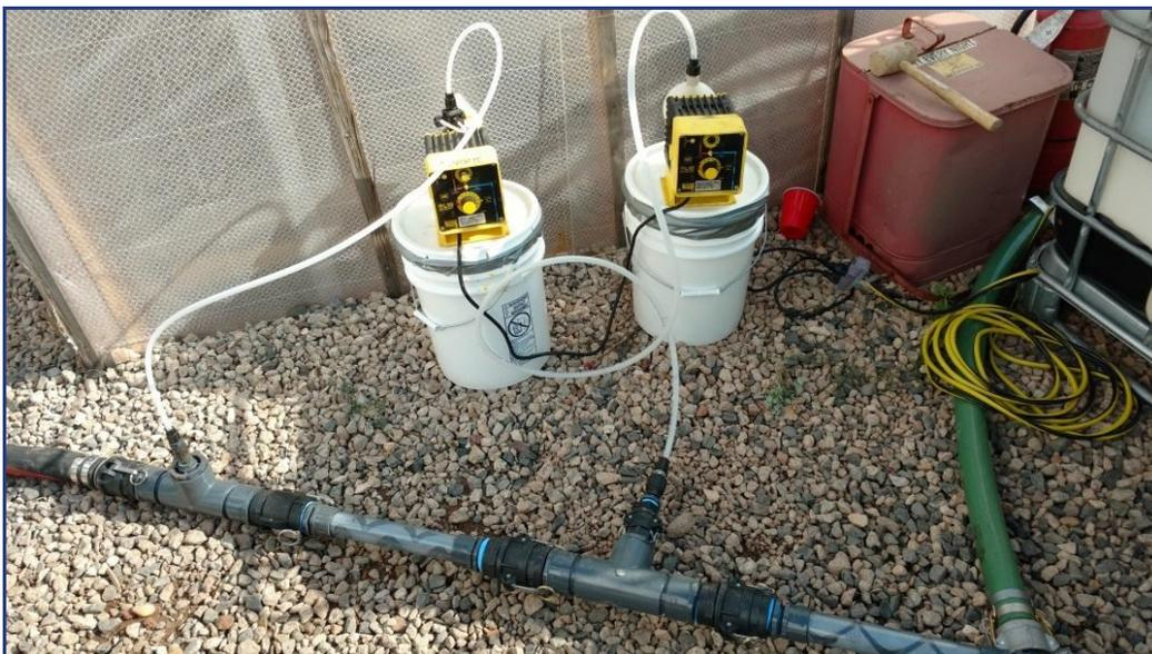
Small metering pumps were used to dose the various chemicals for the on-site pilot study.
