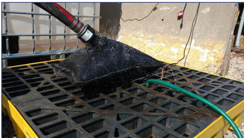
GDT containers were filled with the conditioned solids to simulate a full scale Geotube® container.
