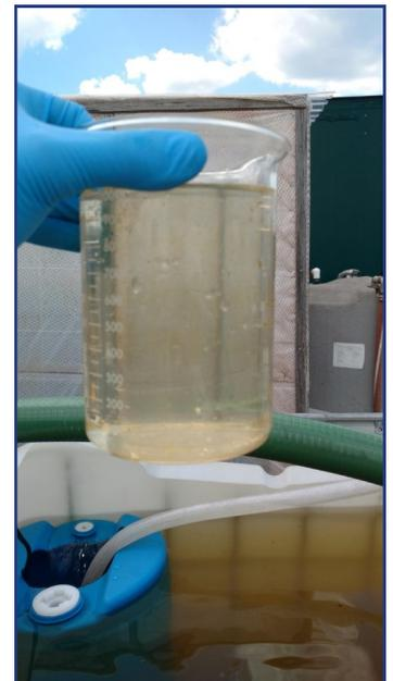
Water samples were collected from several locations during the test. This sample was collected from a tank that was custom built to simulate a weir tank thickening step.
